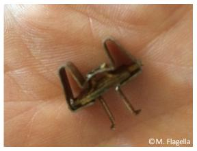
Owner had recently had the altimeter replaced. A technician likely dropped the instrument nut and did not retrieve it after maintenance, causing a short circuit across the Nav light switch from main bus bar.
